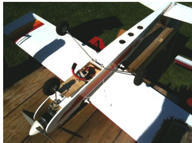
Roger's modifications to convert his Avistar to electric included a hatch to access the battery and cooling holes.
