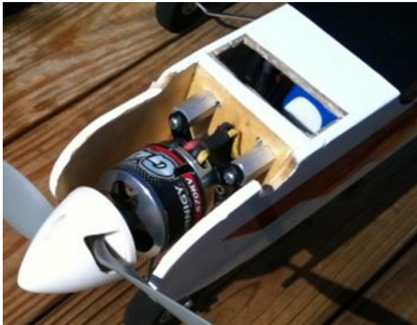
Turnigy 46 electric motor on Roger Mankowski's electric Avistar. Roger is using a 4 cell 5500 mah lipo battery and can get up to twenty minutes of flight time with this set up.
