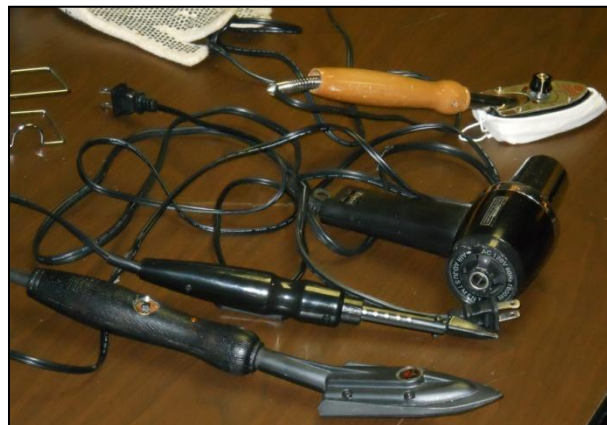
A display of covering tools including a 21st Century Coverite iron with temperature setting knob.
