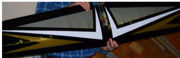
At the November meeting we saw the results of a month of work on the Taurus with the leading edge damage repaired and a four-color Ultracote covering applied.
