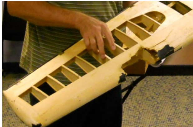
Here is where the club first saw Terry's Taurus project back at our October meeting. Terry had just stripped the wing exposing its big gash in the leading edge.
