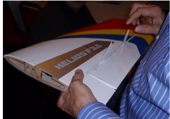
President Les presents his CA hinge secrets to the club--two strips of paper prevent CA mess.
